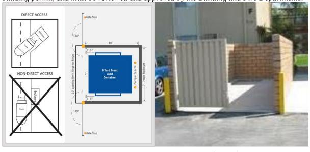
6" dia. pipe bollard, concrete fillled. Set in concrete 3 feet below finished grade, extend 4 feet above finished grade. paint OSHA regulation yellow.
